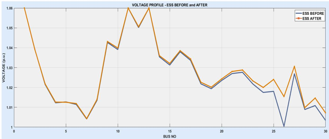
Figure 3. Base case and after-PSO voltage profiles
