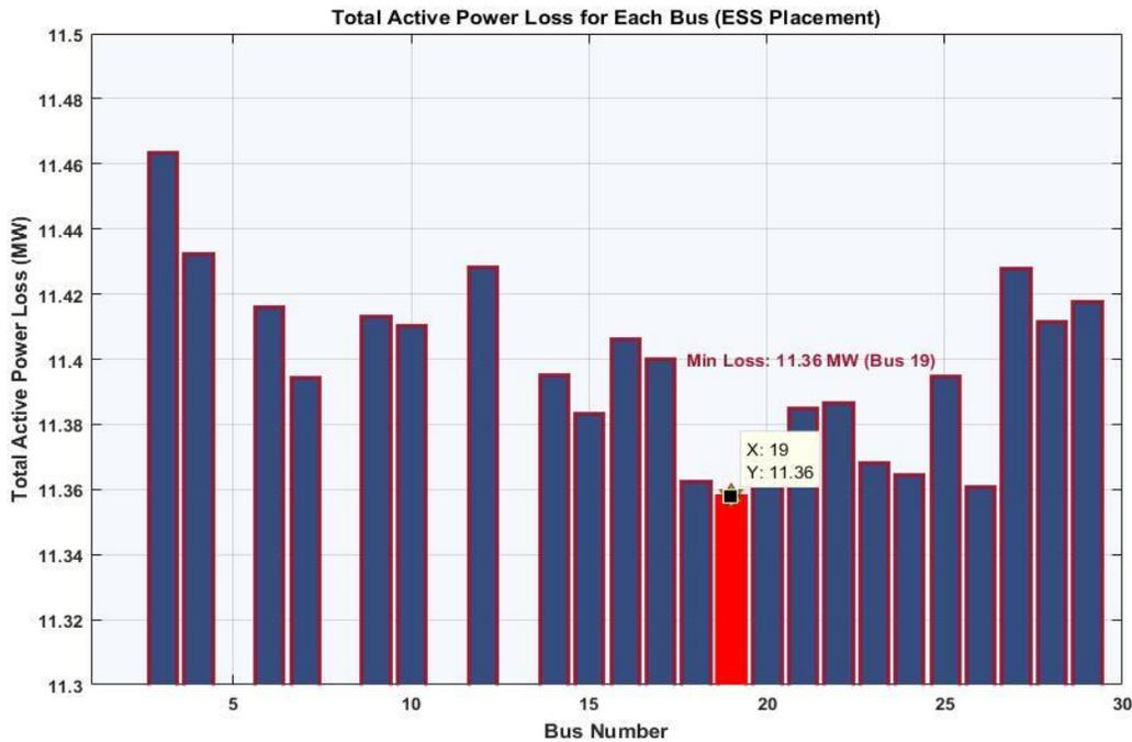
Figure 4. Total active loss after IEEE 30-bus PSO
