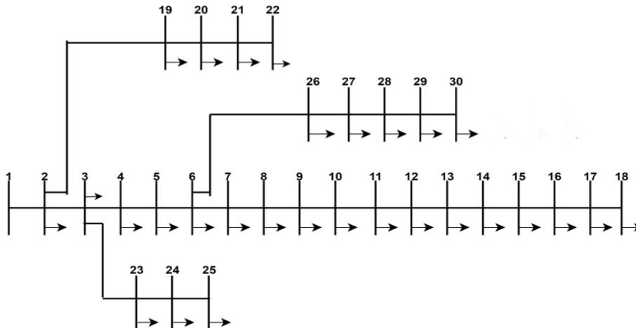
Figure 1. IEEE 30 Bus Power System single line diagram
