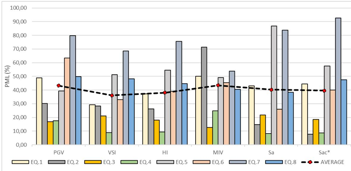
Figure 5. Calculated PML values for different IM parameters
