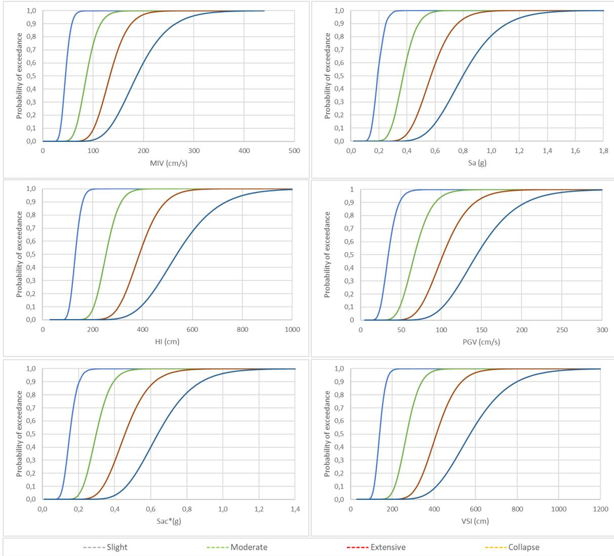
**Figure 4.** Analytically-based fragility curves for different IMs
